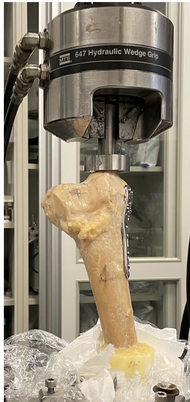
Fig. 3 Depicts the set-up of the biomechanical compression test
